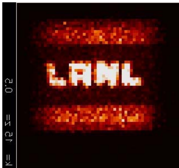
Figure 2. Reconstruction of 1-inch thick lead letters after their exposure in prototype apparatus. Two strips above and below letters are iron bars used as a support for plastic object plate.
